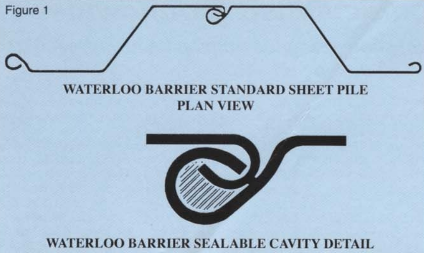
The Waterloo Barrier® system showing interlocking steel sheet piling and modified joint with the sealable cavity.
